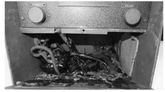
Battery compartment with the microphone, covered with Goo, as received NEW ZEALAND ASSOCIATION OF RADIO TRANSMITTERS
