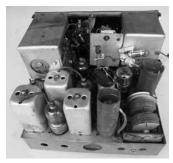
Topside of chassis, showing two VFO shields for RX and TX. The temporary BNC and trimmer, connected to the central aerial spigot, was fitted for transmitter testing.
