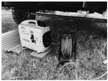
Experimenting with a coiled extension cord as a way to reduce the noise
