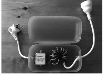
Filter construction; note twisted blue & brown wires.
