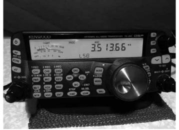
Inverter generator is powering equipment without any filtering; noise is S8!
