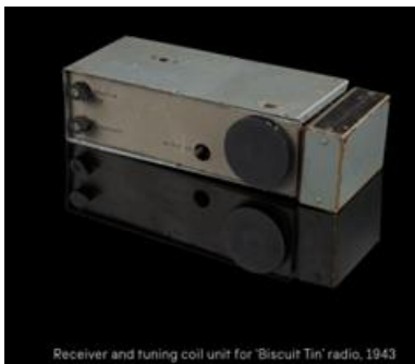
Receiver and tuning coil unit for 'Biscuit Tin' radio, 1943
