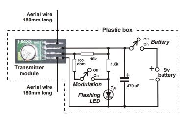
This "test transmitter" is our source of radio frequency energy. It uses a transmitter module smaller than a postagestamp. These are inexpensive and can be obtained by on-line buying on the internet.
