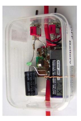
The wires of the transmitter module are splayed out and soldered to the various "lands" in accordance with the circuit diagram.
